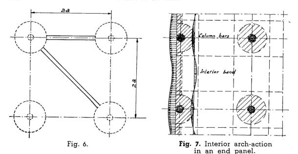
is a continuous floor slab. On account of this, one part of the plate will experience compression (the column bands) and another part will be subject to tensile stresses (the bands running alongside of the columns). This being an internal action the sum of both the tension and compression must be zero. It is rather an intricate calculation to arrive to a reasonable distribution of these compressive and tensile stresses.
