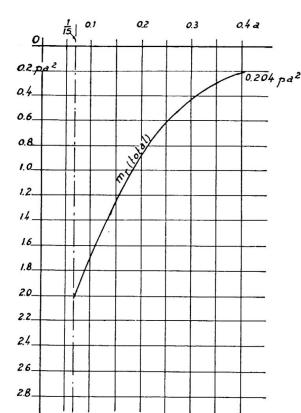
Fig. 5. Radial bending moment in hyperbolical column head.
