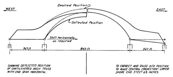
Diagram II. Method of compensating for deflection of cantilevered arch trusses.
