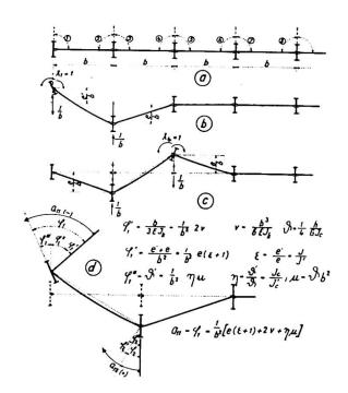
With these designations and with the sign rule indicated on figure 4 and 5 we get the loading quantities and coefficients in the equation system after simplification (omitting the multiplicator  $\frac{1}{b^2}$  in all members):
