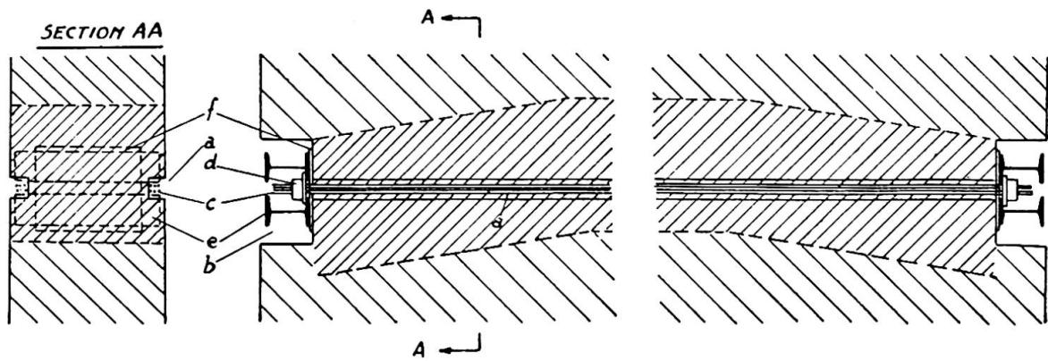
**Fig. 1.** Diagram showing the formation of a prestressed beam in a wall.
