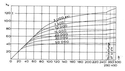
Fig. 5. Effective width of compression elements stiffened along both edges.
