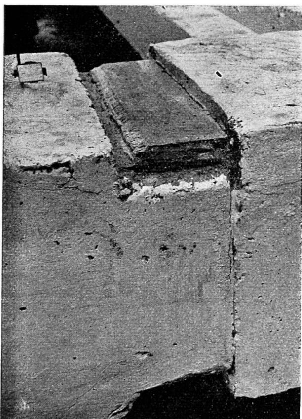
**Fig. 5.** Crack under excess load at welded joint.
