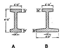
Fig. 2. Girders of types A (partially prestressed) and B (fully prestressed).
