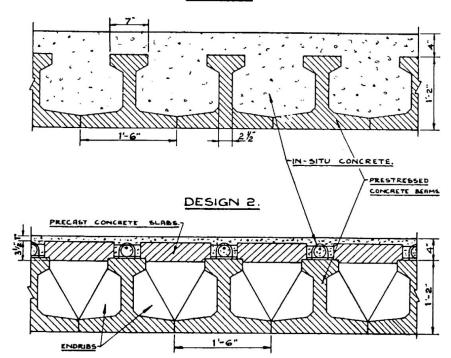
**Fig. 3.** Cross sections of two bridge designs.
