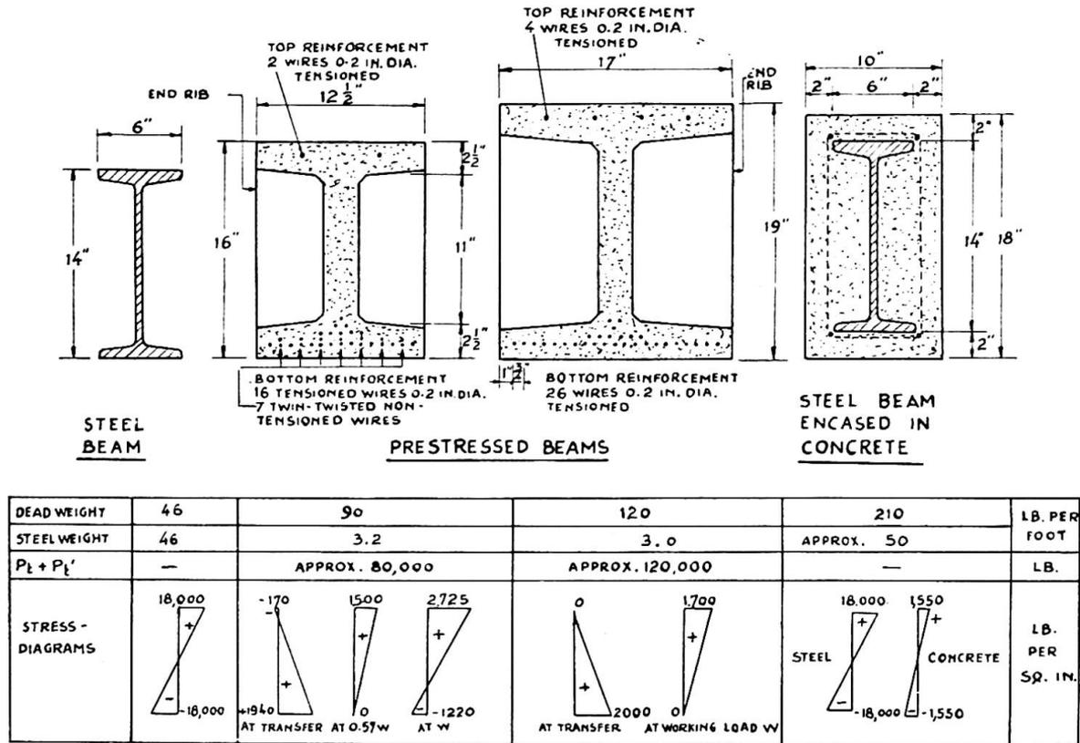
Fig. 1. Comparison of stresses and material consumptions.
