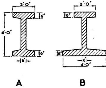
Fig. 2. Girders of types A (partially prestressed) and B (fully prestressed).
