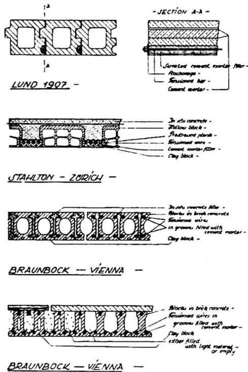
Fig. 4. Development of a prestressed concrete floor construction.
