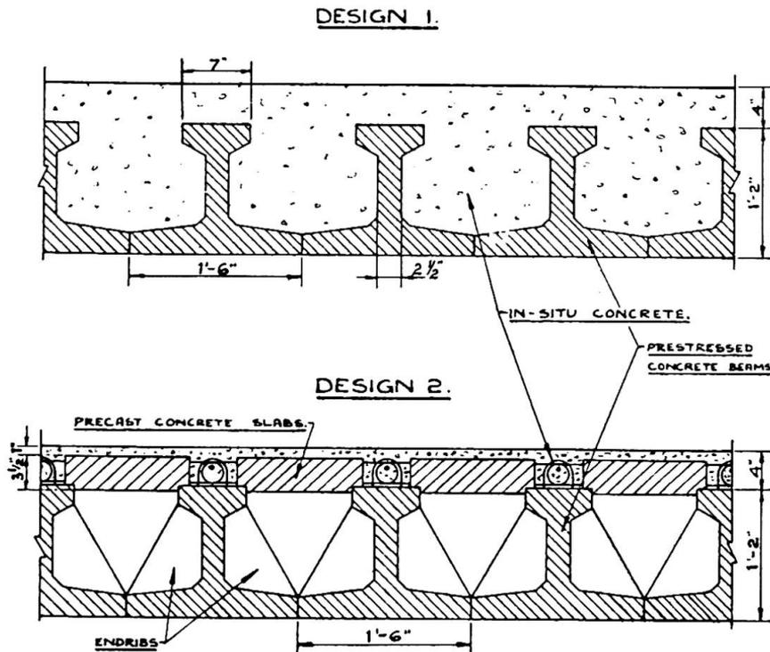
Fig. 3. Cross sections of two bridge designs.
