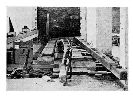
Fig. 5. Prestressed concrete pole under test load 2 100 lb.
