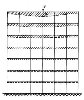
Fig. 1. Estimate of joint movements due to a vertical load on the grid.
