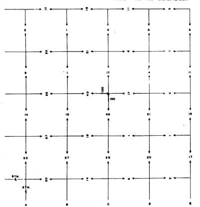
**Fig. 6.** Final direct stresses for one quarter of the gusset plate.
