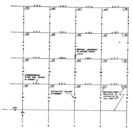
Fig. 3. Estimate of vertical column stresses.
