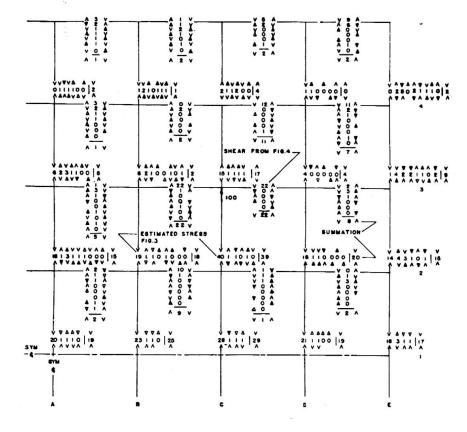
Fig. 5. First vertical force balance.
