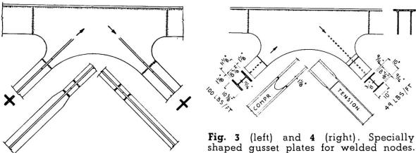
shaped gusset plates for welded nodes.
