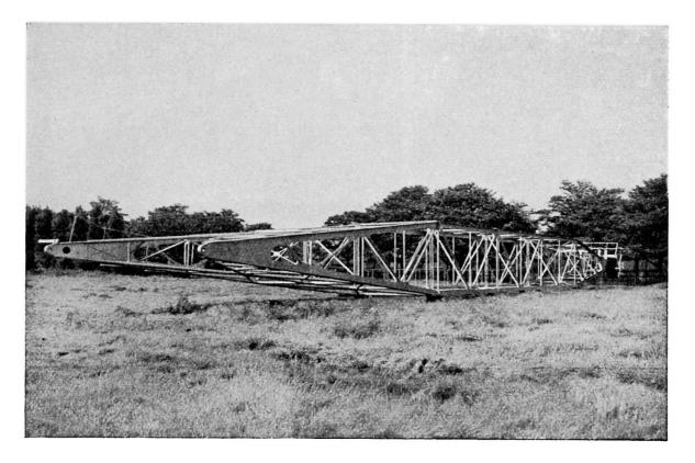
Photo Turners Ltd. Fig. 9. Completed boom prior to its attachment to the machine.
