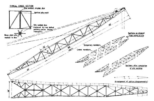
Fig. 6. General arrangement of the welded dragline boom.
