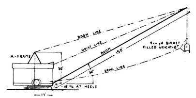
Fig. 5. Diagrammatic sketch of the dragline.
