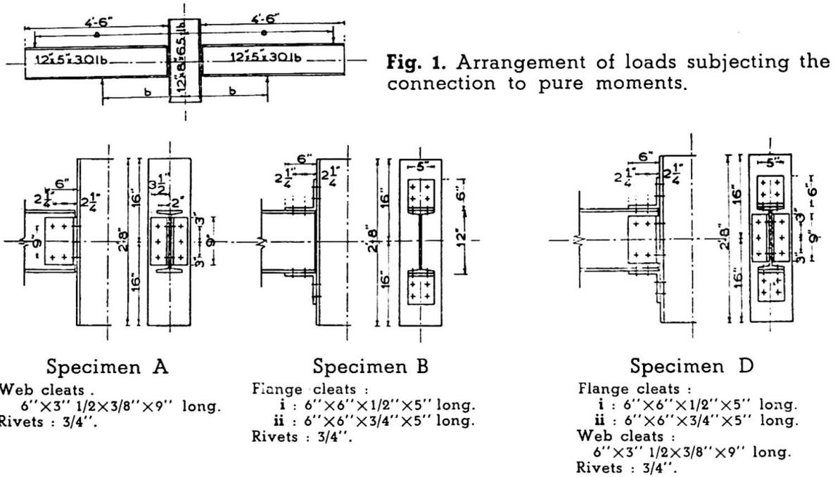
of the latter, while table II, fig. 2, shows the increase in the moments in curve D over those in curve B, expressed as a percentage of the the latter. Table II, therefore, indicates the influence of web cleats on the rigidity of the connection although, in these particular test specimens, the web cleats employed were relatively thin and very shallow.
