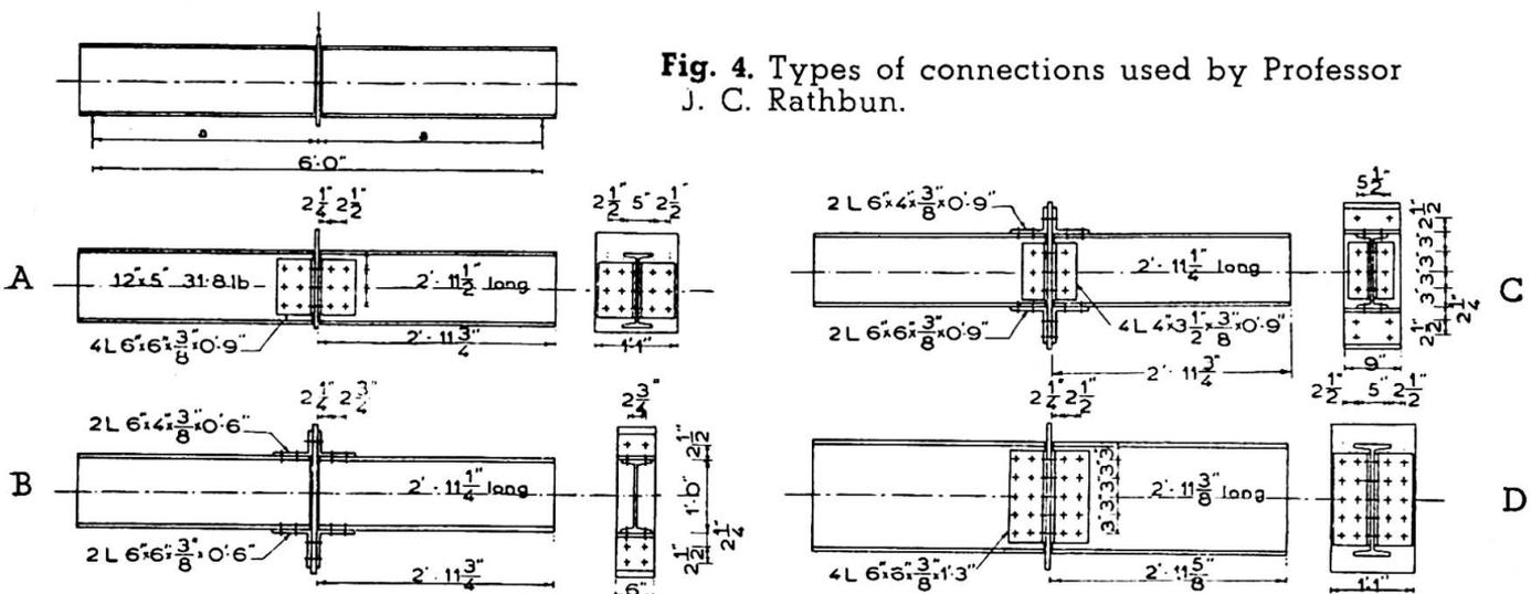
Fig. 4. Types of connections used by Professor J. C. Rathbun.
