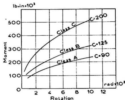
Fig. 22. Standard curves for classified flange cleat connections.
