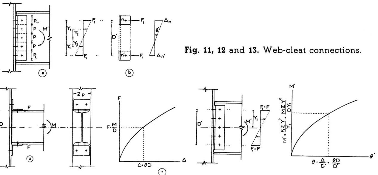
Fig. 11, 12 and 13. Web-cleat connections.
