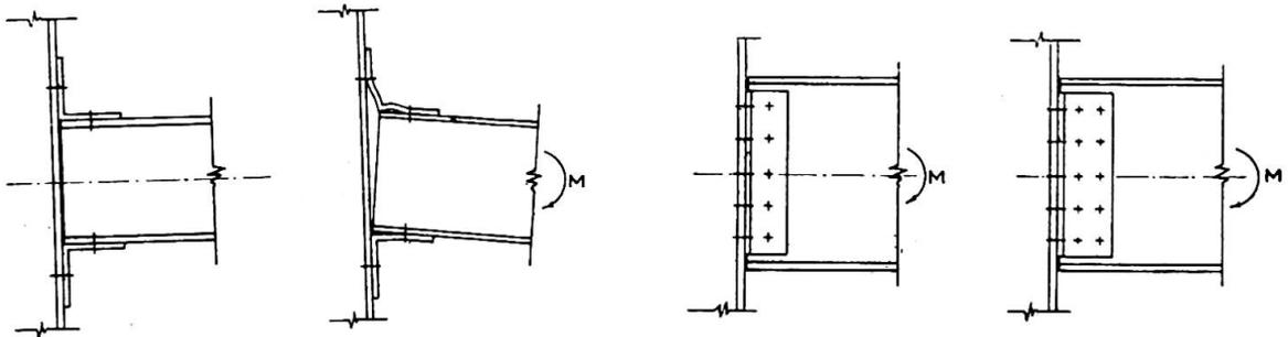
(fig. 7). In both cases, the angles are subjected to a similar pull and will undergo a similar deformation, with the exception that in a web-cleat connection the pull is of varying intensity. In the same way, the behaviour of the compression cleat in a flange-cleat connection can be shown to be similar to the behaviour of the part of the web cleat below the neutral axis in a web-cleat connection under moment.
