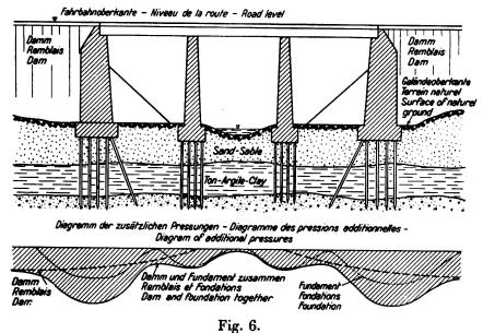
Diagrammatic longitudinal section.
