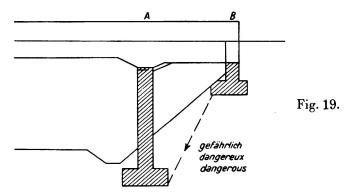
of temporarily reducing the internal angle of friction and therefore of increasing the earth pressure, particularly if the abutment is afterwards set back (Figs. 19
