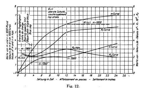
Load test data for Miller road grade separation.
