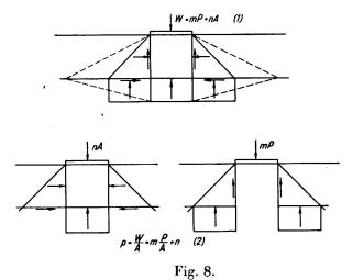
Stress reactions in the linear equation for bearing capacity.
