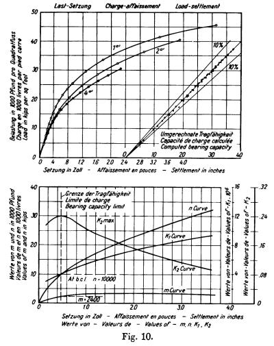
Soil resistance coefficients for incompressible soil.
