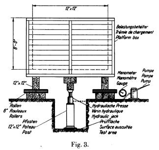
Soil loading test with hydraulic jack.
