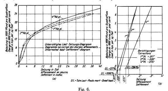
Uncorrected load-settlement diagrams and corrections.
