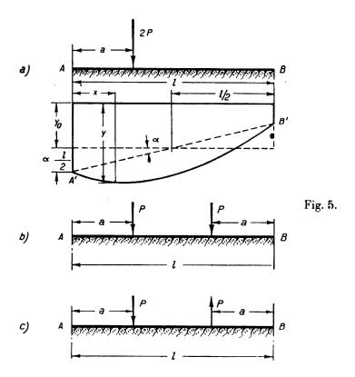
$(y_o=0)$ . Considering the conditions of equilibrium and equating the strain energy of the bar to the increase of potential energy in the foundation, we get,
