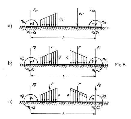
Where  $M'_A$ ,  $Q'_A$ , and  $M''_A$ , and  $Q''_A$ , are moments and shearing forces arising at A from the symmetrical and antisymmetrical loading components respectively, and the F symbols denote the functions shown in Fig. 3:
