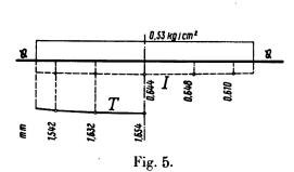
Uniformly distributed load over the layer of rubber. Experimental Qa.
