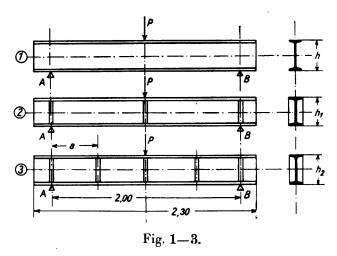
The joists tested were of three types.
