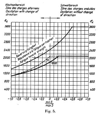
Permissible stresses according to the German Regulations for the Design of Steel Railway Bridges (Heavy Traffic), and tensile fatigue strength of riveted members in St. 52/44. Curve a applies when max S is compressive.
