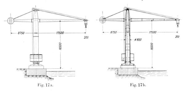
outer one, for reasons of erection, is made in two parts connected by bolted flanges. The same form of connection is used between the two horizontal arms and the upper portion of the vertical member.
