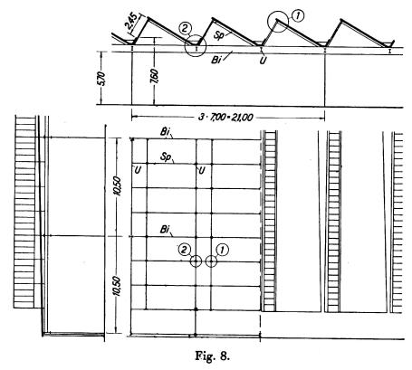
Case A: Supporting rib for bays of  $21 \times 10.5$  m, plate webbed main girder running north and south.
