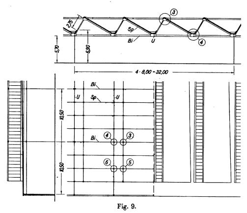
Case B: Carrying ribs for bays of  $32 \times 10.5$  m, main girder of open frame construction running north and south.
