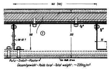
Fig. 13. Light steel floor.
