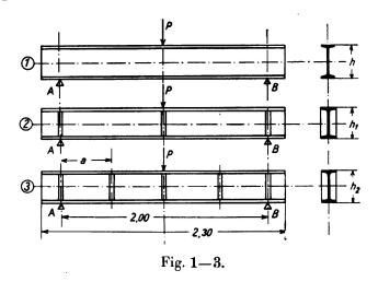
The joists tested were of three types.
