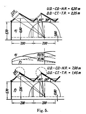
Saw tooth roofs, 7 m — units. T.Q.-Lines for horizontal elements.
