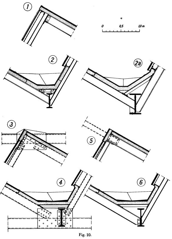
Details of the carrying ribs and arrangement of the roof covering for Figs. 8 and 9.
