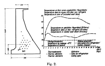
Artificial cooling of the concrete wall of the Allerbüttel double barrage (German Midlandcanal).
