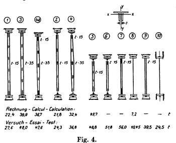
The most important results of calculation and test.
