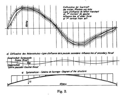
The arch had been investigated beforehand under the assumption that it was isolated, in order to determine the influence line for thrust —
