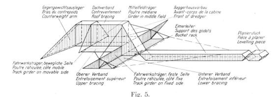
The winding gear and supporting mast of the bucket rack are omitted.
