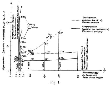
Thicknesses at crown and springings in arch bridges of 250 m span with varying amounts of rise.  $\sigma_{b\,perm} = 100 \text{ kg/cm}^2.$
