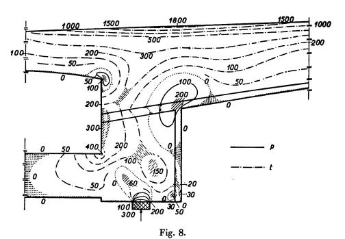
Lines of equal stress v<sub>1</sub> values in t/m.
