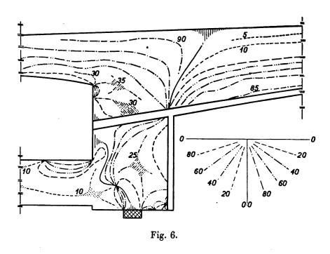
bars, wherever the amounts of tension as determined from Figs. 6 and 7 are in excess of the permissible tensile stresses in reinforced concrete.
