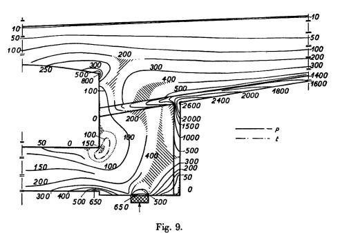
Lines of equal stress  $v_2$  values in t/m.
