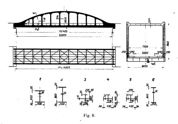
The girder is designed as hyperstatic to the 33<sup>rd</sup> degree.
