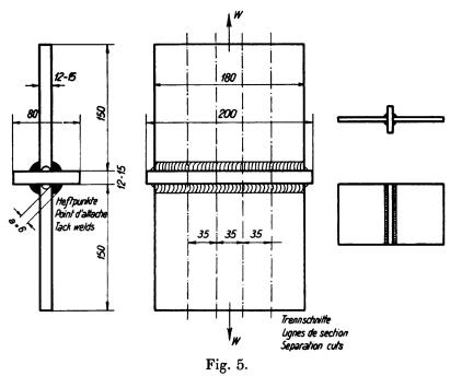
Testing of end fillet welds.
