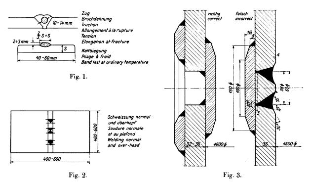
Correct and incorrect closure of place whence specimen has been removed, by welding.
