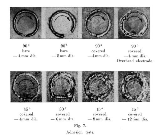
In the testing of finished work non-destructive methods are to be preferred to destructive. The act of weakening the seam by opening it up may indeed have an educational value, but apart from this it should be avoided except as a very rough and ready form of test.<sup>11</sup> The part affected can be rewelded, but in doing
