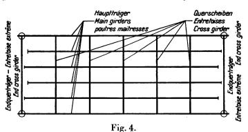
Shrinkage of main girders of a grated bridge.
