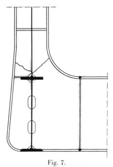
Characteristic cracks in uprights of Vierendeel bridges.
