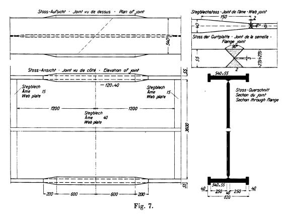
spanning over 5 openings of 54 m each. After accurate measurements carried out by the Staatliches Materialprüfungsamt in Dahlem a welding procedure was laid down which called for pre-stressing to approximately 300 kg compression in order to reduce the maximum tensile stresses due to dead and live load at the
