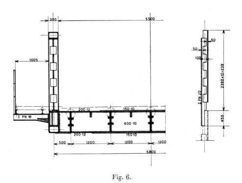
obtained and then welding the two projecting portions. The floor of the bridge consists of rolled beams of the well-known "Alpha" type, covered by a reinforced concrete slab.
