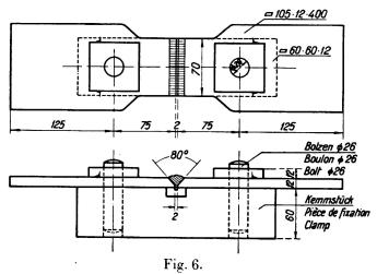
Arrangement for measuring shrinkage stresses.
