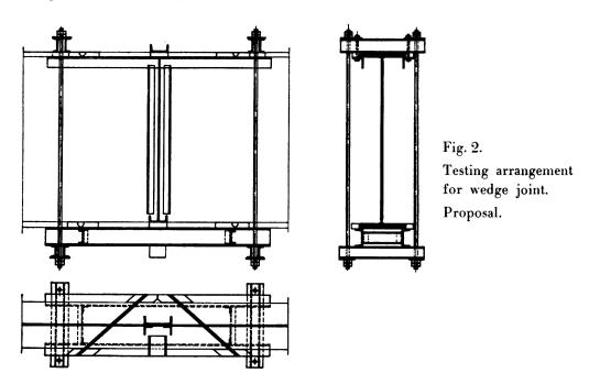
two-thirds of their total dephth a powerful angular contraction occurred, which had to be counteracted by continually tightening the clamping on the parts to be joined. Fig. 2 shows the design of a clamping arrangement, and Fig. 3 in-
