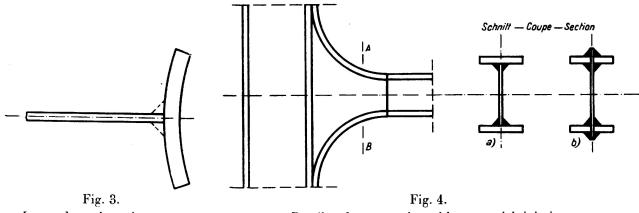
Inverted camber given to a welded plate.
