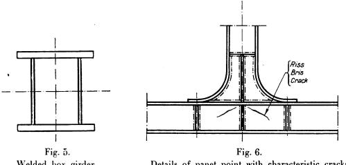
Welded box girder. Details of panet point with characteristic cracks.
