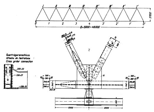
Fig. 11. Main girder. Intersection No. 1.
