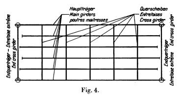
Shrinkage of main girders of a grated bridge.
