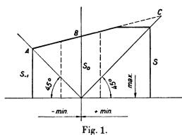
at B, min = 0, and the ordinate  $S_o$  is the unit stress selected to be permitted in the case of pulsation from zero.
