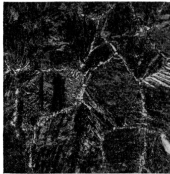
Not pre-heated, formation of Martensite.
