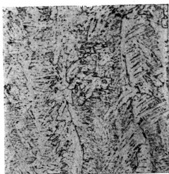
Coarse Widmannstaetten structure in weld metal.
