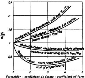
Fig. 5. Relative increase or decrease of different limits of strength for increasing peak stress (form coefficient  $a_{kr}$ ).
