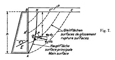
hypothesis of plane rupture surfaces, for an arbitrary arrangement, of the direction of E, leads of course to contradictions in the equilibrium of forces in the slipping earth prism, for which reason *H. Müller-Breslau*, *H. Reissner* (l. c.) and others found it necessary to calculate with curved rupture surfaces. The main problem — the ascertaining of the form of the rupture surfaces requiring the greatest earth pressure E to ensure equilibrium — has not been solved up to the present time.
