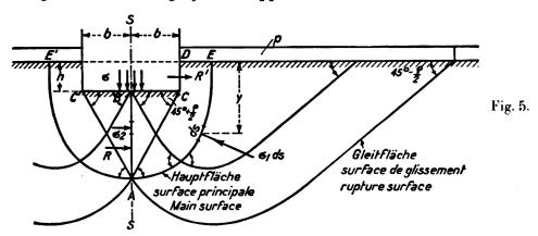
stressing at the limit of equilibrium. The specific compressive stress of the foundation we shall designate with  $\sigma$ , and we shall assume that outside the foundation there also acts a surface stress p.
