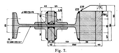
Marcinelle Lock Details of suspension for Stoney sluice
