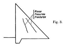
be traversed not only by two vertical cro sed fissures, but also by a horizontal fissure encircling the block mid-high. This phenomenon is easily explained. Shrinkage took place more rapidly towards the surface. Since the centre core did not contract to the same extent, it put the outside in tension and caused it to crack.
