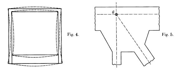
The verticals are subjected to bending moments in a plane normal to the girder, and these cause tension on the inside and compression on the outside face. As the vertical is normally in compression, it is easy to understand that the mean stress  $E_1=1.12$  in the case of instruments 1-2 placed on the outside would be larger than the mean stress  $E_1=0.88$  measured by the instruments 9-10.
