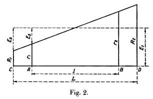
Knowing the measured values of stresses  $r_1$  and  $r_2$  at the points A and B separated by a distance l (Fig. 2) the mean stress in the member has been calculated; this corresponds to the stress due to the principal force and has the value
