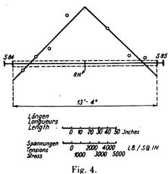
Observed stress due to torsion when a central concentradet load of 8.1 tons was applied to Beam No. 840 D.
