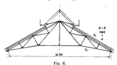
Roof construction for the Power Station Engerthstrasse of the Municipal Electric Works, Vienna.
