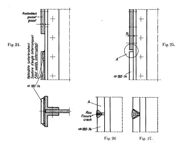
thin fillet weld, the gap A was merely welded over (Fig. 26). This weld cracked at one point.
