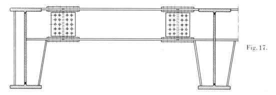
Cross beams and frames may be butt-welded to booms which are subjected to compressive stresses only. (See Fig. 18.) When welding booms subjected to alternating efforts — such as may be found over the supports of continuous
