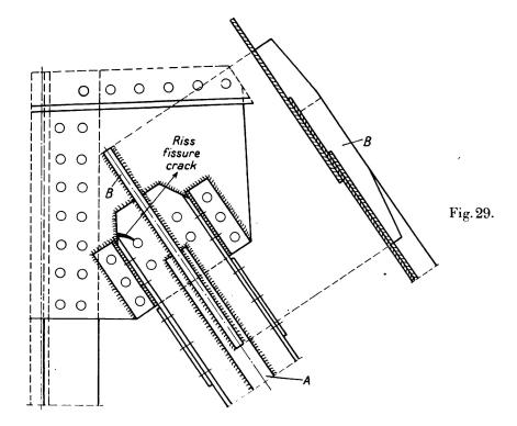
nection because the member is subjected to stress resulting from the weight of the bridge itself. The shrinkage stresses due to welding cannot be easily determined because Hook's Law no longer holds good for plastic material on account of the change of the modulus of elasticity, and so the actual conditions governing tension are very far from clear.
