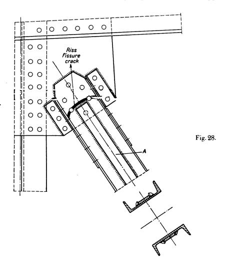
May 1931. Flat bar iron reinforcing straps A, welded on both sides of the webs of channel section iron terminated behind the previously countersunk rivet of the connection (Fig. 28). It was thought that the connection had been sufficiently reinforced according to the calculations which had been made by connecting the end of the member and the angle irons to the gusset plate by fillet welds and by welding the projecting leg of the angle iron to the projecting flanges of the channel section iron.
