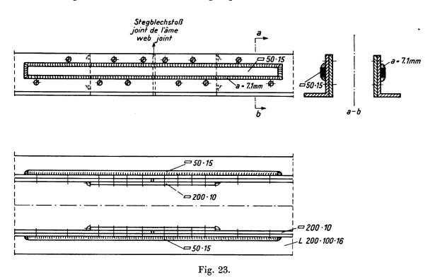
ating stressing up to the permissible stress as would be the case with a new bridge. Present-day experience goes to show that the reinforcement straps which have been welded to the web would have to be carried into the panel points. The reinforcement could be slightly improved by machining the ends of the side fillets and the end fillets in order to produce a smooth and gradual transition from weld to plate. But even so, and in the most favourable circumstances, the
