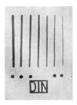
Fig. 2.X-ray picture (positive)of wire screen Cu II.
