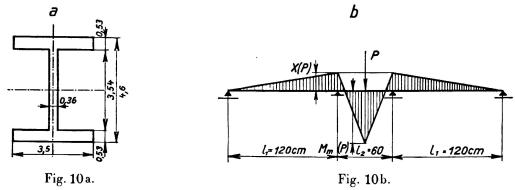
Cross section und loading arrangement of the test beam used by Stüssi and Kollbrunner.
