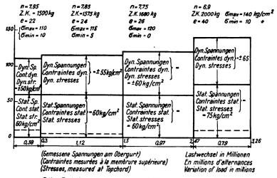
Z.K. = Zentrifugal-Kraft - force centrifuge - centrifugal force
