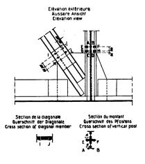
Effort principal calculé dù à la surcharge seule: Diagonale A-C:- 2.83 kg/mm² Diagonale B-D:- 3.27 kg/mm² Diagonale B-D:- 3.27 kg/mm² Berechnete Hauptspannungen infülge allein der Yerkehrslast: Diagonale A-C: 2.83 kg/mm² Diagonale B-D: 3.27 kg/mm² Calculated Stresses due to external loadings only: Diagonal member A-C:-2.83 kg/mm² Diagonal member B-D:-3.27 kg/mm²
