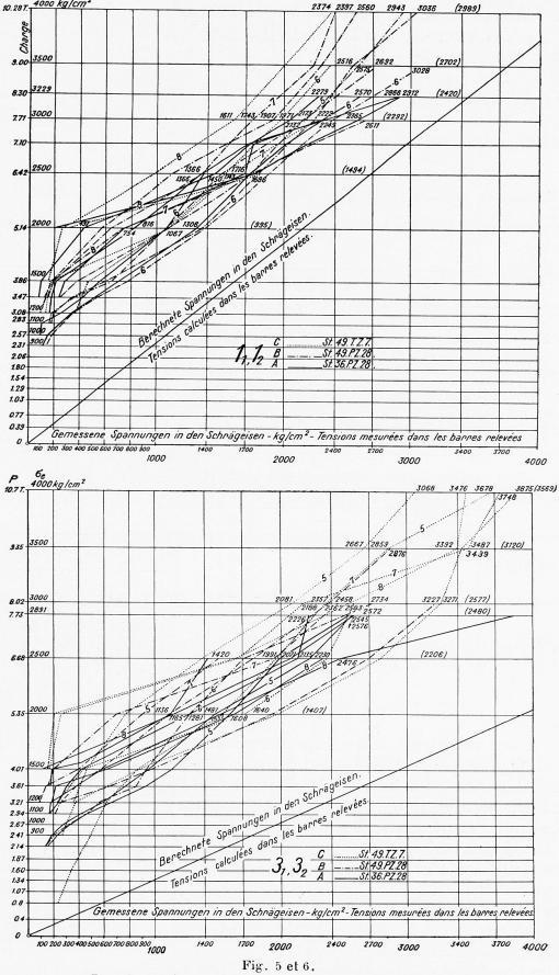
Berechnete (gemessene) Spannungen in den Schrägeisen = Calculated (measured) stresses in the inclined bars.
