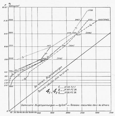
$\label{eq:Fig.7.} \mbox{Fig. 7.} \\ \mbox{Berechnete (gemessene) B\"{u}gelspannungen} = \mbox{Calculated (measured) stresses in the stirrups.} \\$
