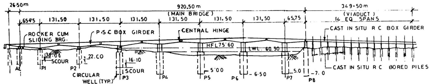
**FIG. 2 GENERAL ARRANGEMENT OF BRIDGE**
