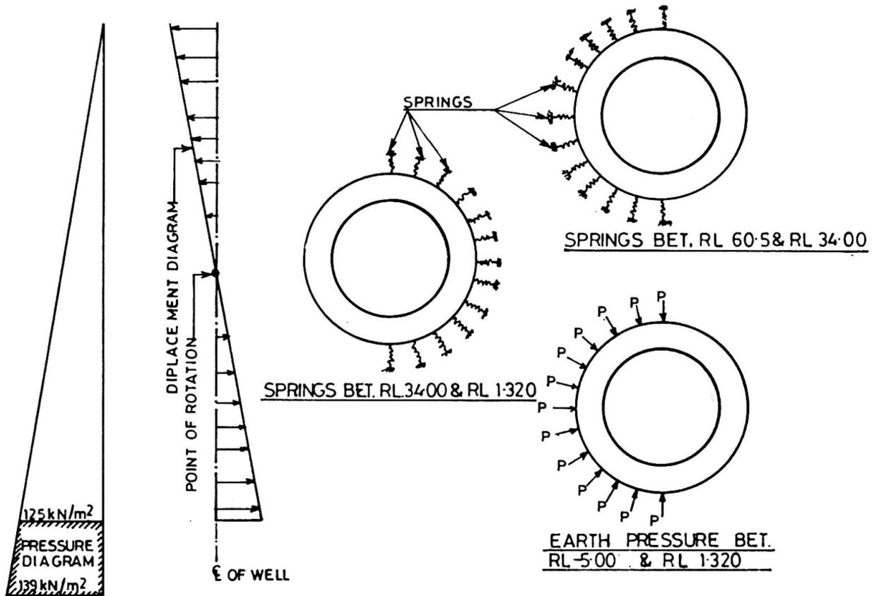
FIG-4 SAND BLOW CONDITION - APPLIED FORCES AND DISPLACEMENT MODEL
