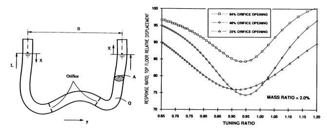
Fig. 1 A typical liquid column tube
