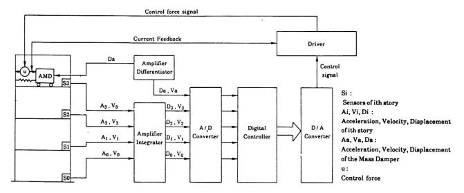
Fig. 3 Active Mass Damper System
