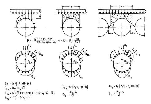
Fig. 2 Load assumptions for earth surcharge
