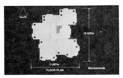
Fig. 3: Floor plan of Brick Castle with tendon location.
