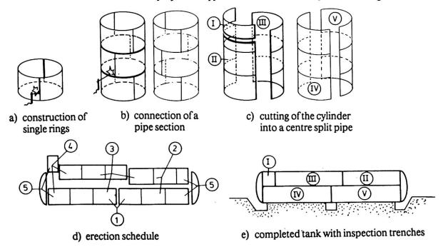
Fig. 6 Assembling course for the split pipe method
