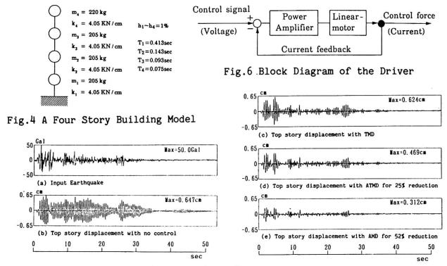
Fig. 5 Active Control of the 4 Story Building Model
