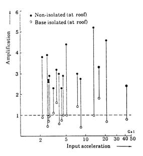
Fig.2 Ovserved Amplification of Acceleration Response.
