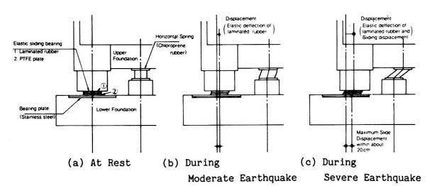
Fig. 1 Composition and Isolation Mechanism of TASS System
