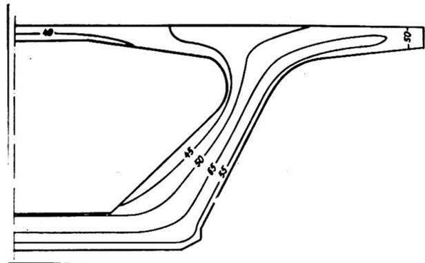
Fig.2 Temperature field in the middle section of a segment-match (isolines values are given in °C)
