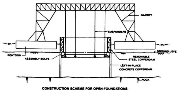
Fig.6 Detail of floating gantry with cofferdam assembly
