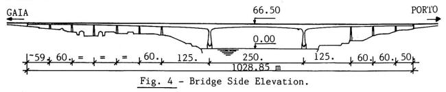
The grandiose  $\pi$  - shape portal with a continuous girder over the supporting piers has a 250 m. long main span and 125 m. long side spans. On the left bank (Gaia) approaching side, the girder has one 58.85 m and five 60.00 m long spans
