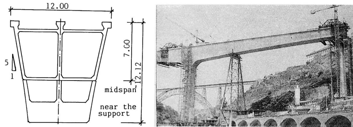
a. Girder Cross Section. b. Temporary Steel Frame Shoring.
