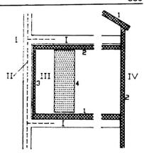
Ad 3. The connections between the building components are divided into five categories: remote (no direct relation), touching, connected, meshed and unified. In this sequence, five levels of integration are indicated.
