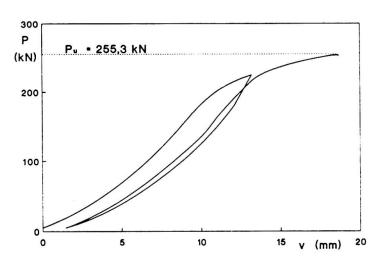
Fig. 2. Mid-span deflection versus load.
