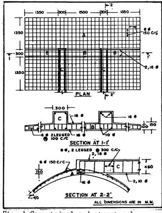
Fig. 1 Geometrical and structural details
