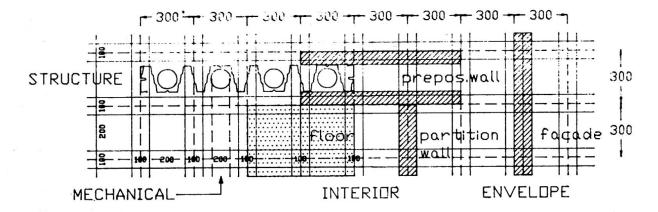
Ad 2. the building sequence of the three finishing systems: interior, envelope and mechanical, is also prescribed by scenario alterations for guaranteed flexibility in use and with different lifespans of the building components in mind. Accessibility of the piping systems is important in this respect.
